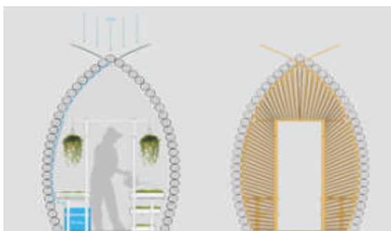
Figure 39: Rain Water Collection (Arch Daily 4)
